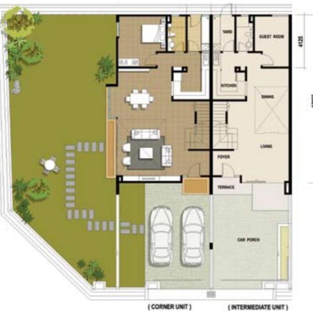
Typical 3 storey terrace units - Ground floor plan.
